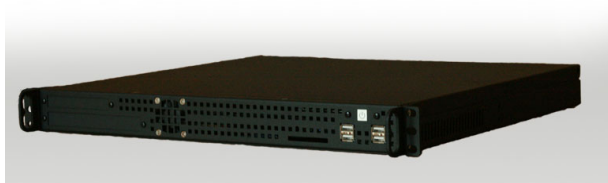
Figure 1: QtProxy server in RACK 19"1U casing
